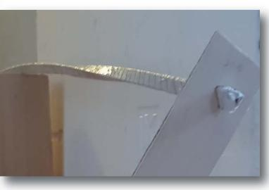
Figure 4 : Twisting of the triangle beam (here with thespiral wrap)
